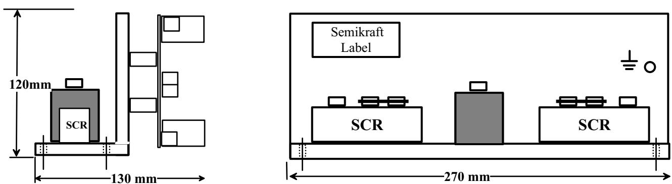
**AI-L270 0,90°C/W AI-L270(F) 0,3°C/W (F) means cooled with extern Fan not in ouer delivery.**
